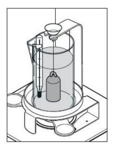
Add the liquid whose density you wish to determine to the beaker (up to approx. 1 cm above the suspension eye of the sinker). Ensure that no air bubbles adhere to the sinker (remove any air bubbles with a fine brush).
